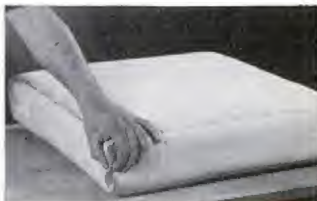
Above, strips of solid slab rubber are cemented to edges and at four corners of built-up center portion
